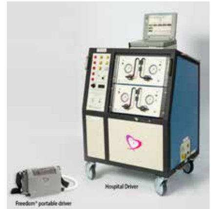
The 13.5 lb Freedom® portable driver and the 418-lb “Big Blue” hospital driver
